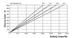
Weight of caliper and lever assembly - 10.62kg Weight of lever assembly only - 1.4kg Maximum Braking Force = 8.3kN @ 0.9kN force on lever
