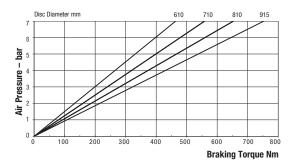
Maximum Pressure 7 bar Maximum Braking Force = 1.9kN @ 7 bar Weight of caliper and thruster - 9.52kg Weight of thruster only - 0.3kg Volume displacement of thruster at full stroke = 64ml
