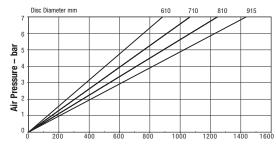
Maximum Pressure 7 bar Maximum Braking Force = 3.6kN @ 7 bar Weight of caliper and thruster - 10.37kg Braking Torque Nm Weight of thruster only - 1.15kg Volume displacement of thruster at full stroke = 150ml
