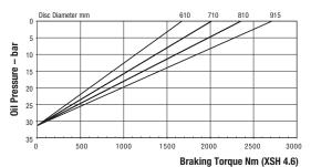
Maximum Braking Force XSH 4.6: 6.8kN Minimum Pressure for full retraction: 40 bar Weight of caliper and thruster - 13.22kg Weight of thruster only - 4kg Volume displacement of thruster at 6mm retraction = 9.1ml
