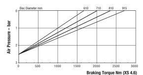
Maximum Braking Force XS 4.6: 6.8kN Minimum Pressure for full retraction: 3 bar Weight of caliper and thruster - 13.72kg Weight of thruster only - 4.5kg Volume displacement of thruster at full retraction = 1.19 l
