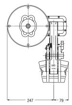
Maximum Braking Force = 6kN Weight of caliper and actuator - 17.9kg
