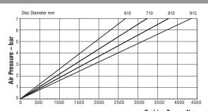
Maximum Pressure 7 bar Maximum Braking Force = 11kN @ 7 bar Weight of caliper and thruster - 11.28kg Braking Torque Nm Weight of thruster only - 2.06kg Volume displacement of thruster at full stroke = 426ml
